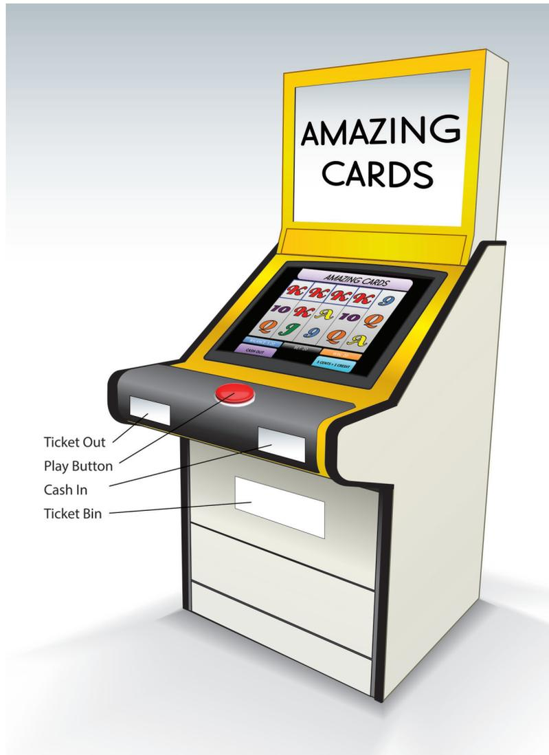
*Figure 2.* A schematic representation of a TapTix machine.
